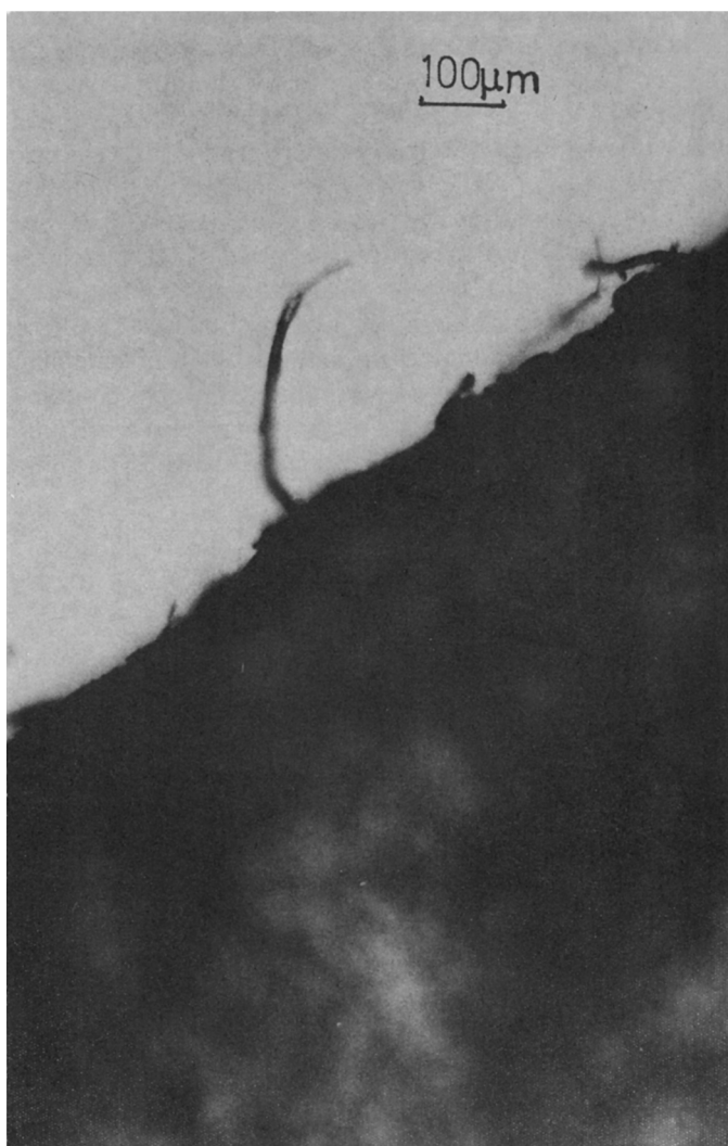
Fig. 9. Isolated fiber on the fracture surface of sample A.
